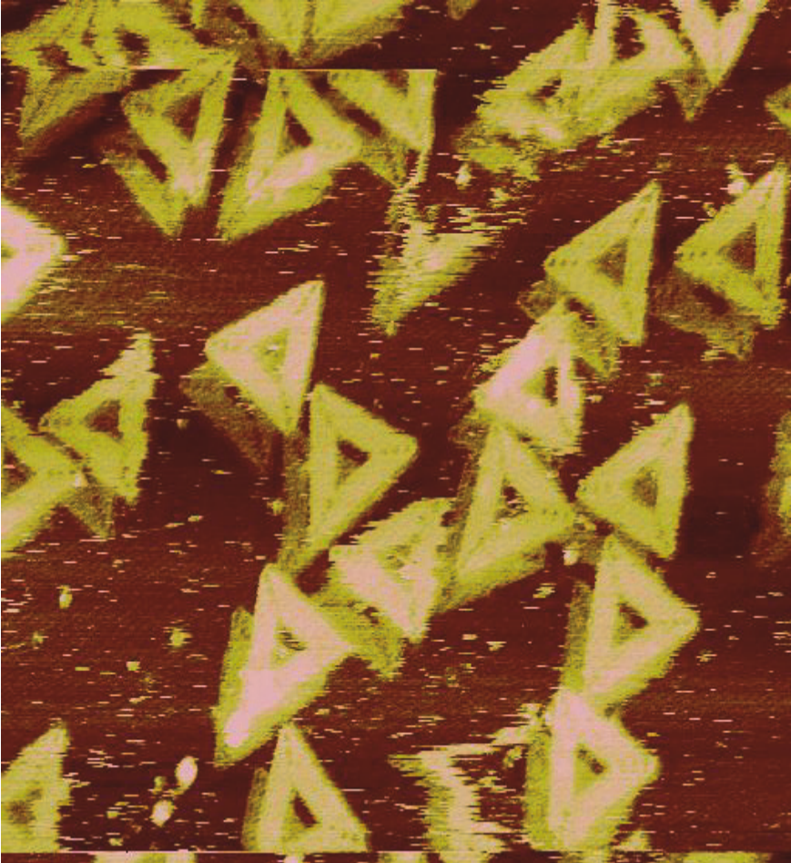
Figure 4. AFM image of triangular scaffolded DNA origami on a freshly cleaved mica surface. Image size 1 \times 1 \mu\text{m} , height 2nm.
